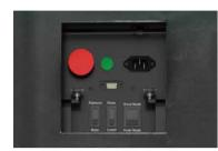
A lower operation panel is designed to enables the operations such as operation platform lifting, brake release, etc. to be performed outside the vehicle so as to facilitate vehicle maintenance.
