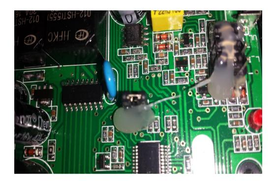
Please Note If the control unit is to be exposed to moisture once fitted to a vehicle i.e. Quad, Motorcycle etc it will need to have a cover fitted to avoid the ingress of dirt and moisture.
