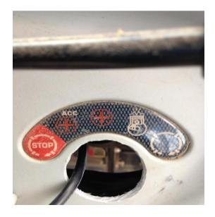
Thread the button wiring through the hole. Bend the securing tabs on the back of the button to fit through the hole, once in place reach behind the button and bend the tabs back out to secure the button in place. The RFID reader can now be threaded over the START/STOP button wire and held in place behind the button with a suitable bonding agent (this will also ensure that the button cannot be easily removed).
