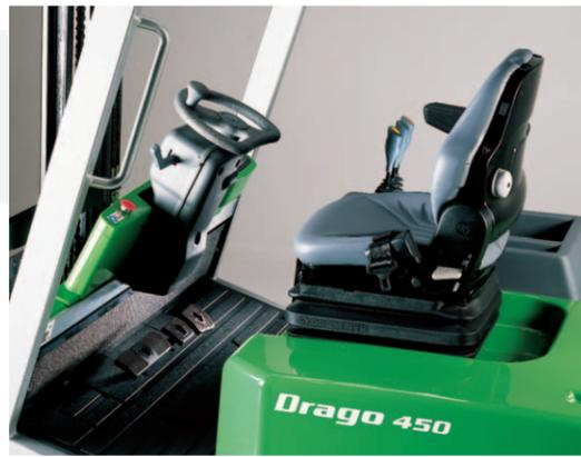
Space for the operator. The cab provides wide space to the driver and a clear view when manoeuvring. The truck may be fitted with pedal direction control to suit all driving styles.
